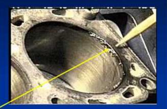
Sludge and Carbon build-up
