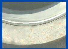
Crankshaft Main Bearings looked like new, there were no traces of wear. They maintained their original coating. Usually after 17,000 hours they are chewed up. In this engine we used **Polytron**, so there was almost no wear at all after 30,000 work-hours.
