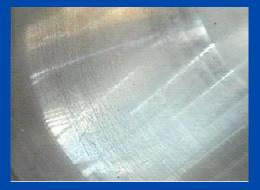
Cylinder liner from our 30,000 hours old engine with **Polytron MTC** totally clean with almost no wear at all.
