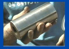
After 30,000 hours in operation and 100 hours in the presence of water, all the piston pins didn't have any traces of wear, looked polished-like and new.
