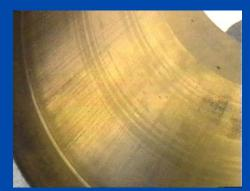
Piston-rod bearing from 16,000 hours old engine, (without **Polytron MTC**) chewed up as a result of wear
