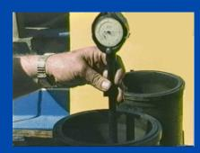
There was almost no wear on the liners and the dimensions were within the manufacturer's specs.
