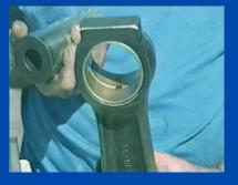
After 30,000 hours in operation and 100 hours in the presence of water, all piston pin bearings didn't have any wear and looked like new.
